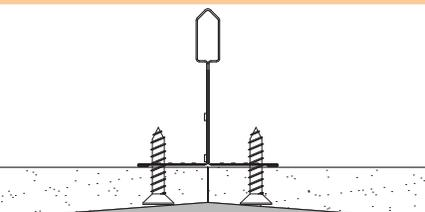
Factory tapers on all 4 edges of GypSorb Stratum panels. Joints are taped and filled with standard joint tape and compound.
